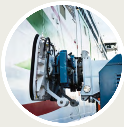
Taking advantage of the latest technology: The automooring system of West Terminal 2 also reduces air emissions.
